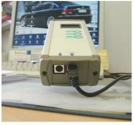
brightness of flat panel monitors and flat panel displays. It calculates the light power observed by the human eye in candela/m<sup>2</sup>. This cd/m<sup>2</sup> unit is also known as Luminance.
