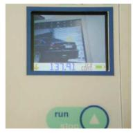
The instrument is portable and weights 450g only, which make it simple to use. Just orient the front of the instrument to the monitor under investigation. The measured value is spontaneously displayed in  $cd/m^2$ . The Figures above are of the instrument oriented to a flat panel monitor with a photo of a car as the background. The instrument is measuring the color of the rear of that car.
