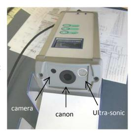
accurate measurement can be obtained when the instrument is at 50 cm from the monitor and at the normal to the monitor surface.
